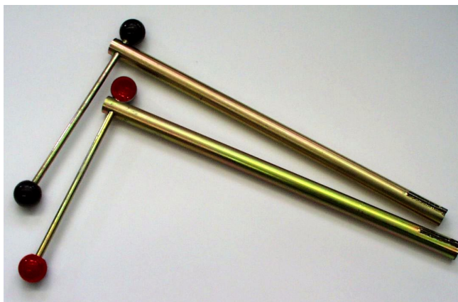
Fig. 39: Rotary lever: with red head for earthing and de-earthing; with black head for closing or opening the switch-disconnector
